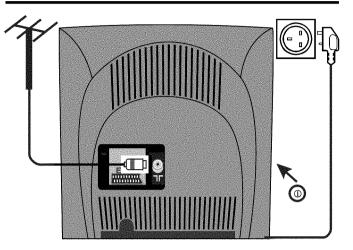
1 Insert the aerial plug into the  $\neg \neg$  socket.
